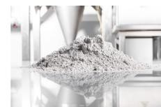
**VESTAKEEP® 4000 FP** is an unreinforced, highviscosity polyether ether ketone fine powder. It can be used as a basic resin or in blends with different additives for manufacturing compression molding parts.
